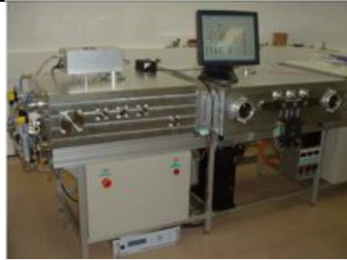
KAI-M, large-area industrial reactor, 40x50 cm 2 VHF (40.68 MHz)
